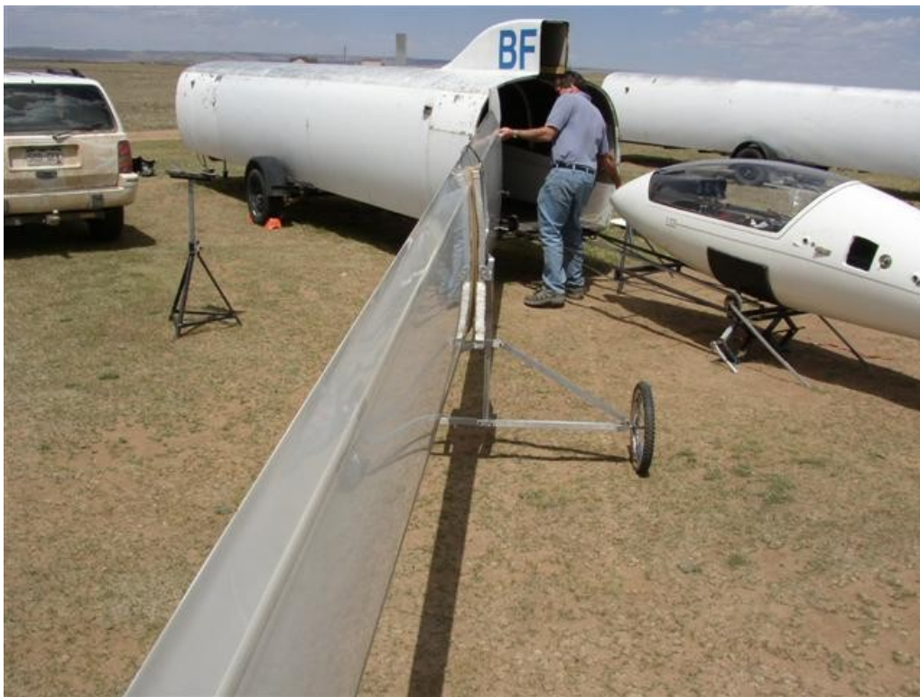
The root dolly vertical lock is unpinned.
