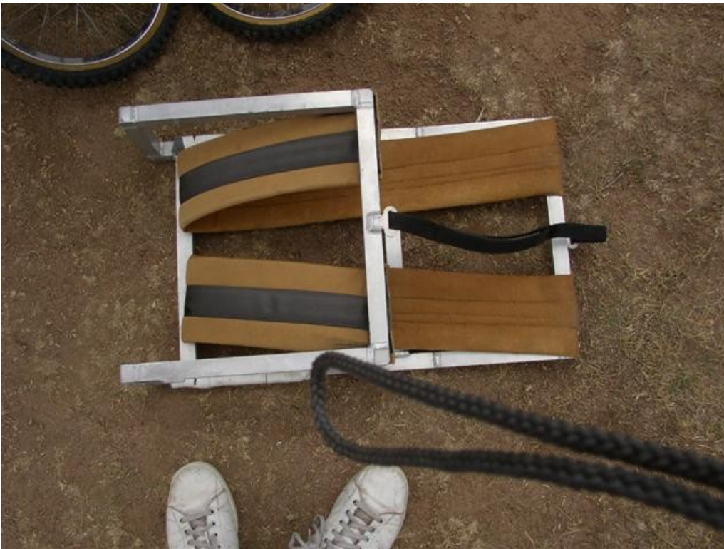
The strap fits through a loop and Velcro secures it to itself. The wings tend to stay flat when rotated flat. My Udo dolly tends to be forward loaded and the wings tend to want to stay vertical. At the balance point, the LAK chord is two inches wider than the LS-3. The LAK panel is 47lbs heavier than the LS-3 and about 3m longer.
