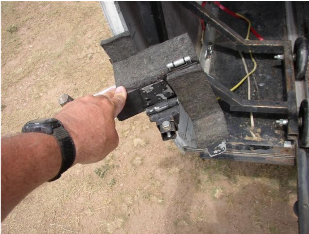
The root dolly is hinged at the lock, and for rotation.
