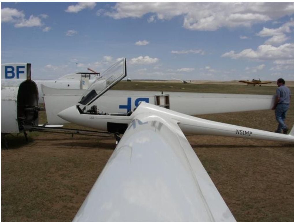
Right wing is extracted.
