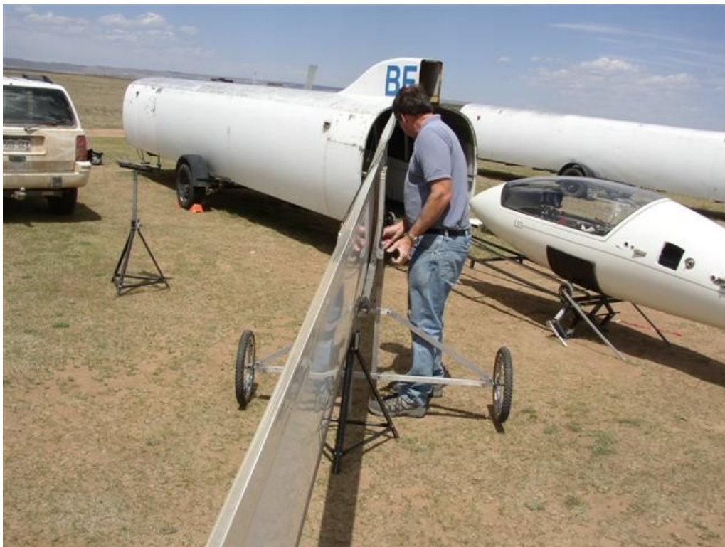
The dolly is attached to the saddle and the wing stand removed.
