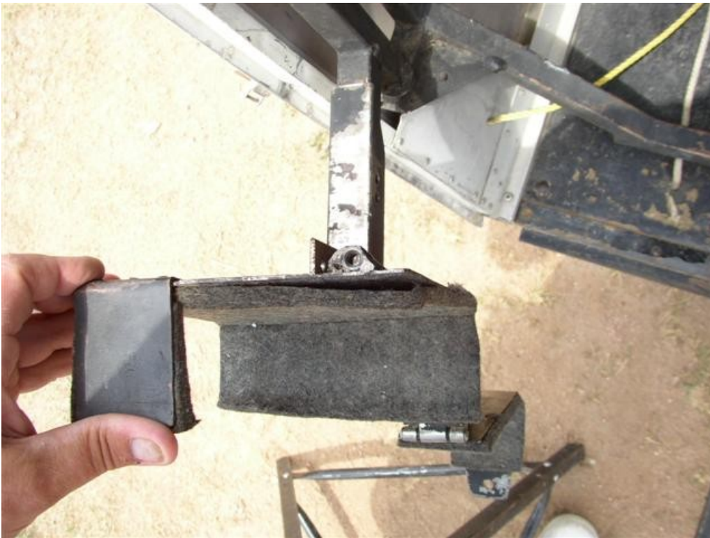
These pivot as a unit to allow the wing to swing.
