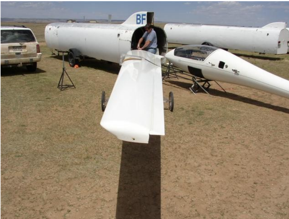
The wing is rotated, then the spar lock is released. Note the wide track of the dolly. This can be done single handed in winds to 25kts.
