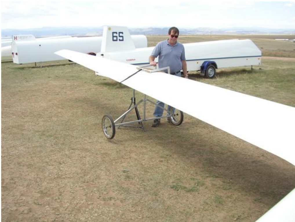
Wing stand is placed and dolly removed from saddle. Note wheels are a couple inches above ground.
