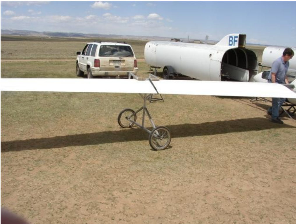
The root is jockeyed into position.
