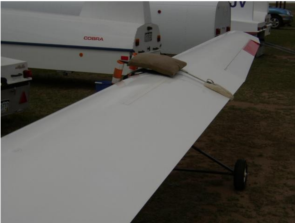
This saddle uses an adjustable strap and plastic latch. I think I like the Velcro method better.
