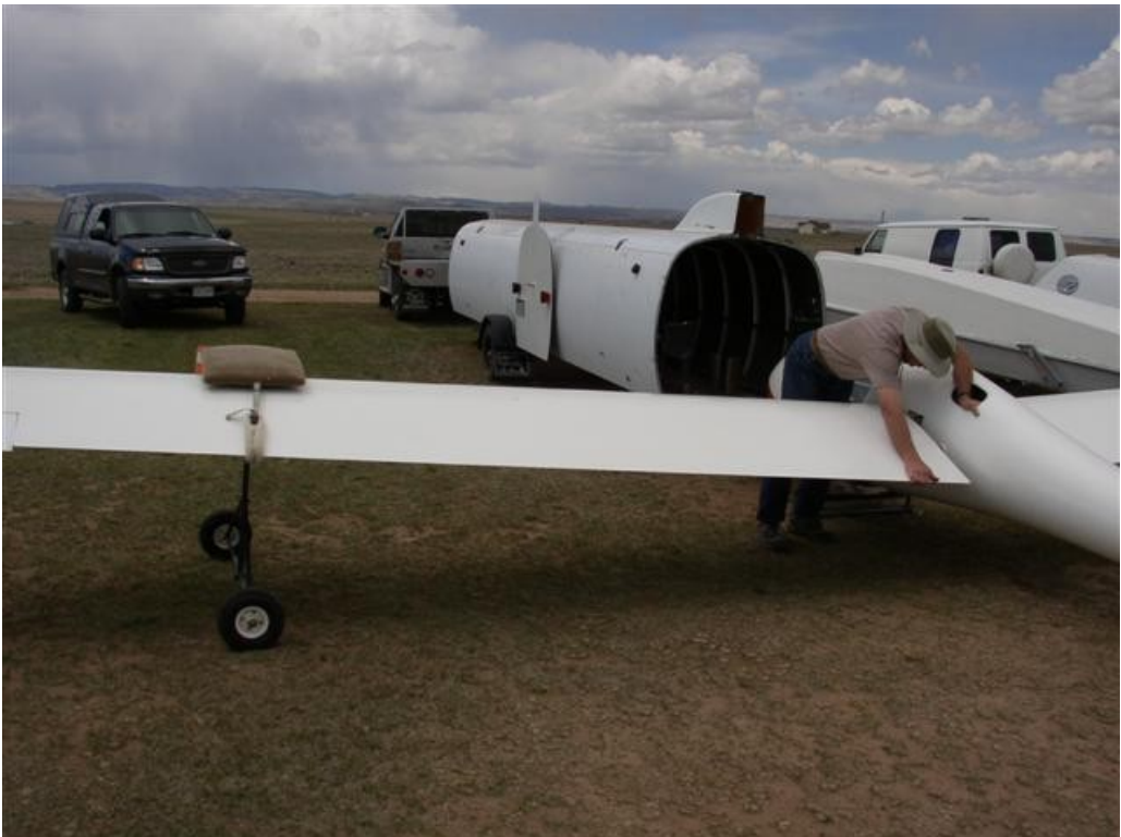
Lifting both leading and trailing edges of the G102 is the trick to get the locking pins home.
