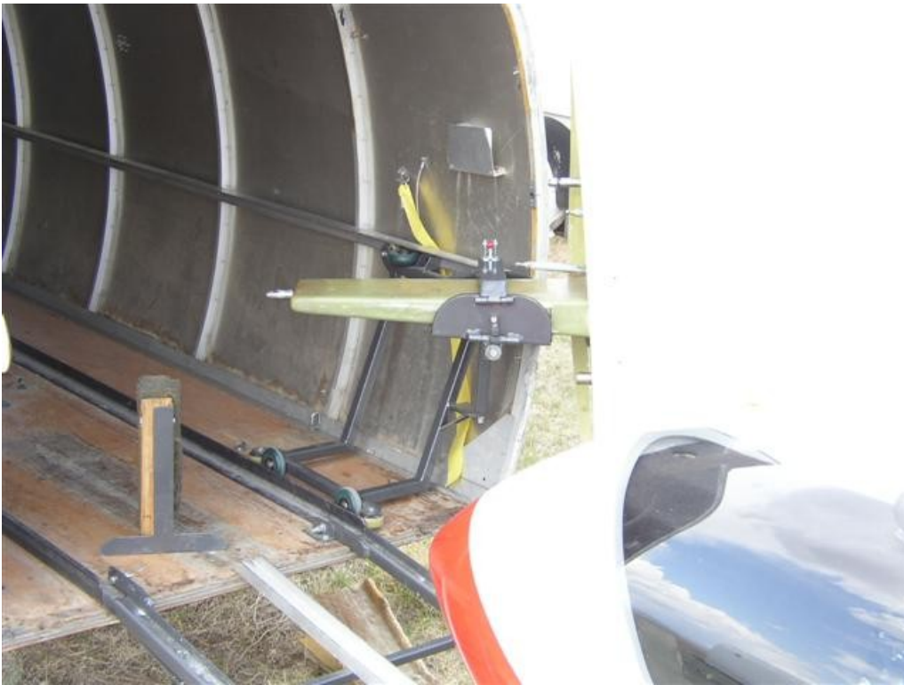
Root dolly, wing pivoted. All steel has been powder coated. Trailer tip stand standing in rear of trailer.
